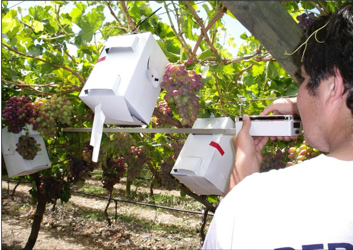
Figures 3.6 Light penetration into the vineyard canopy was measured with a ceptometer on a weekly basis.
