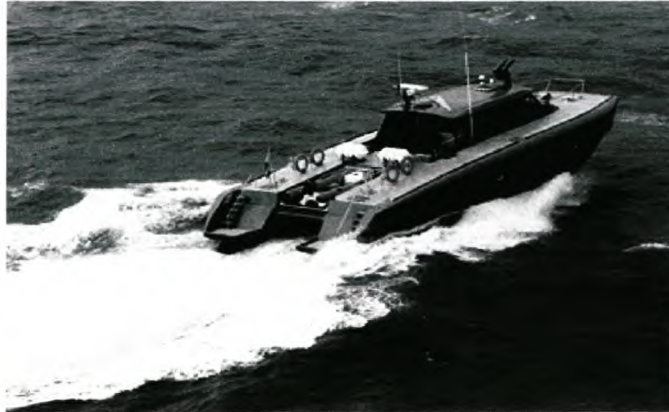
Figure 1.4: A 22m coastal patrol catamaran using a Hysucat hydrofoil system. The vessel is capable of 36 knots.
