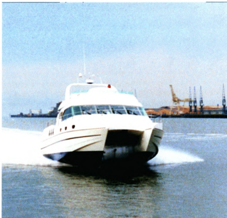
Figure 6.1: A Prout catamaran with a Hysucat foil system and an asymmetrical hull design
