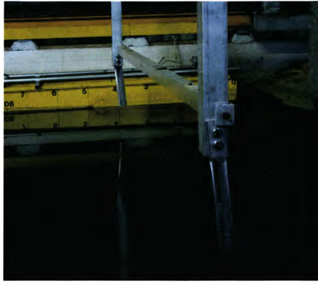
Figure 3.9: Arrangement of wires for turbulating the freestream ahead of the model
