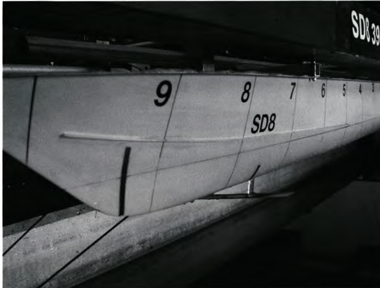
Figure 3.1: Spray rails for a Hysuwac model. Also shown are the turbulence stimulators on the hull (black strips).
