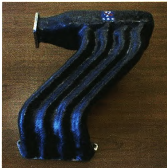
Figure 9-7. Prototype Inlet Manifold
