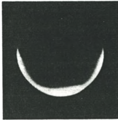
Figure 2.8: Typical visual characteristics of Hermstein's glow discharge [6].
