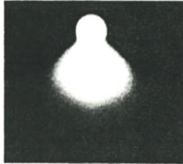
Figure 2.5: Typical visual characteristics of a pulseless glow discharge [6].
