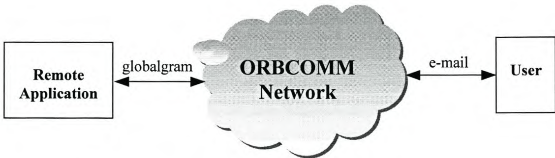
Figure 5-1 ORBCOMM Network Inputs and Outputs
