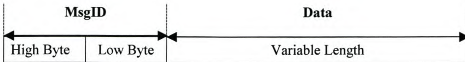
Figure 3-7 Layer-to-Layer Message Structure
