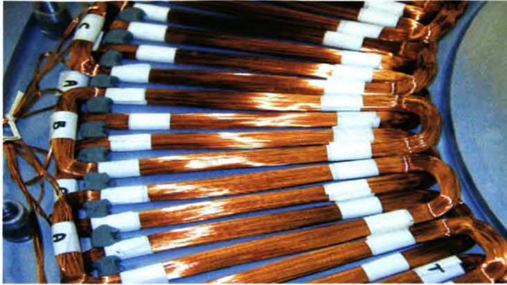
Figure 4.2: View of the stator coils in the former.
