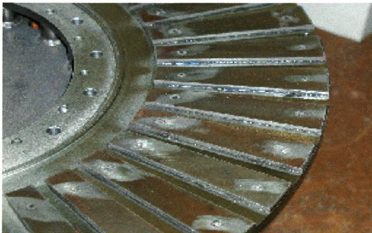
Figure 5.14: Rotor magnets with pins inserted.
