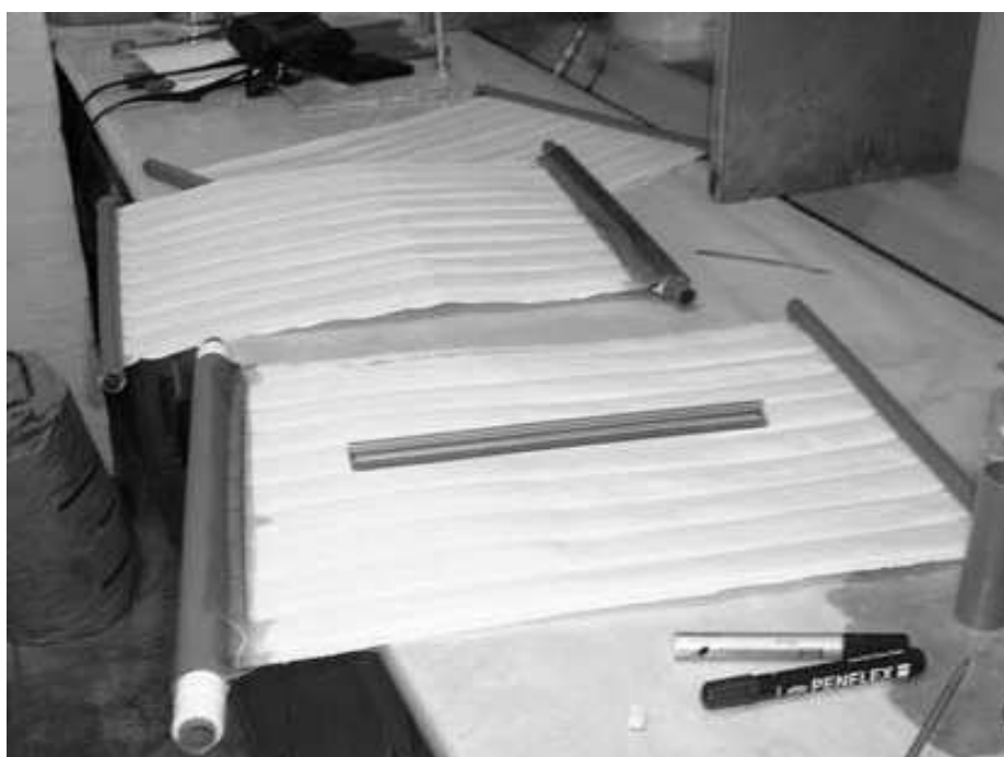
Figure B.1: A photograph of three membrane elements under construction.
