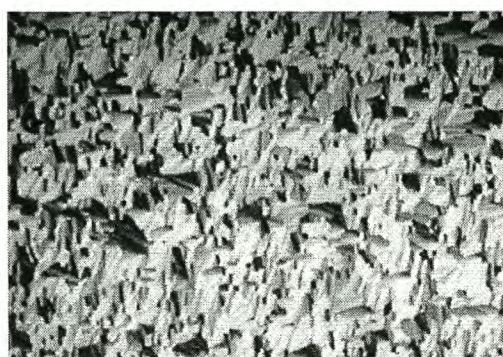
Figure 5.5b Developed phases (about six hours old)
