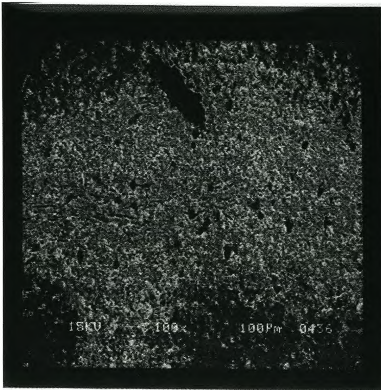
Figure 1.5 Typical image of high star-like particle concentration
