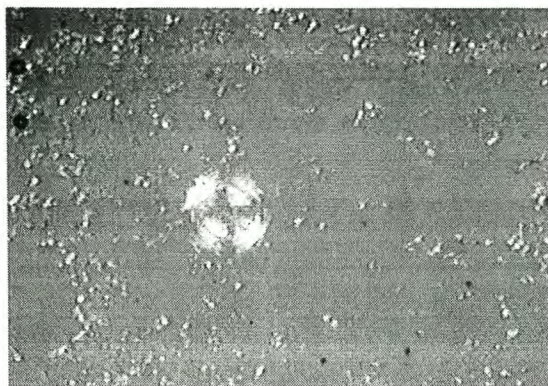
Figure 5.4 Undeveloped phase (Immediate image of sample with 10% monomer and 45% surfactant after irradiation)
