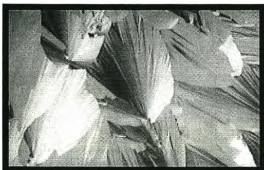
Figure 5.2a Fan-like structure of the hexagonal phase
