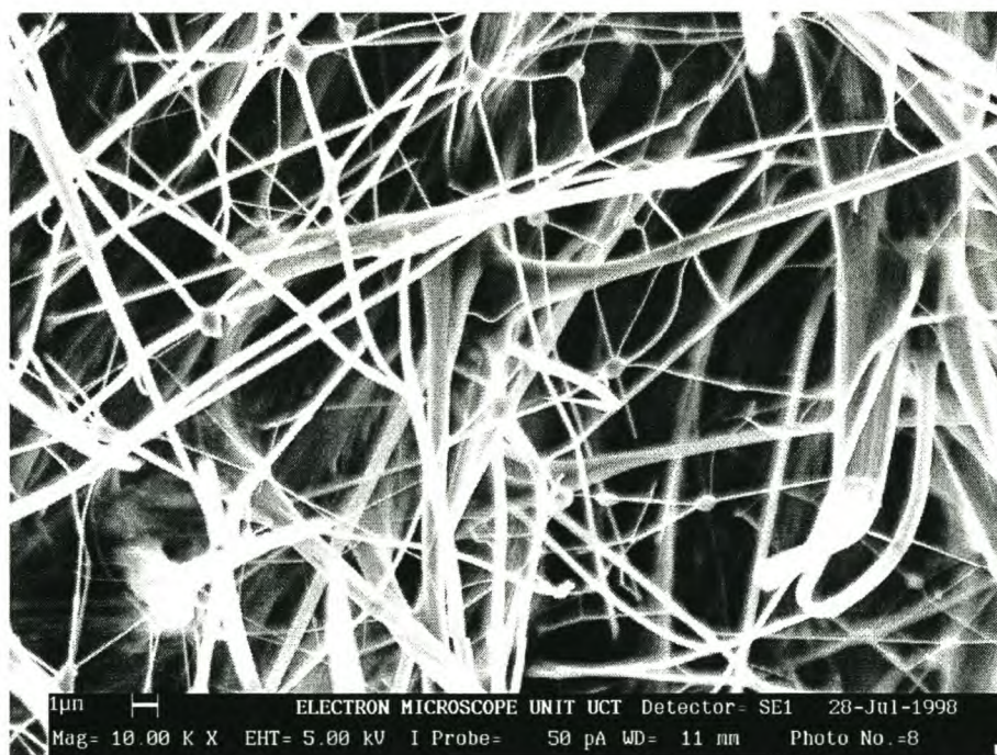
Figure 2.8 Surfactant gel showing “cold drawing”
