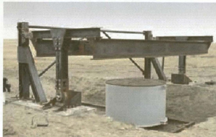
Figure 2.4: Canadian Centre for Mine Action Technologies (2006) apparatus for the measurement of blast effects from larger buried charges. Rating 2 kg C4. Total load is measured with four large force transducers.
