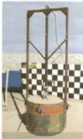
Figure 2.3: Canadian Centre for Mine Action Technologies (2006) apparatus for the measurement of blast effects from small buried charges. Rating 100 g C4.
