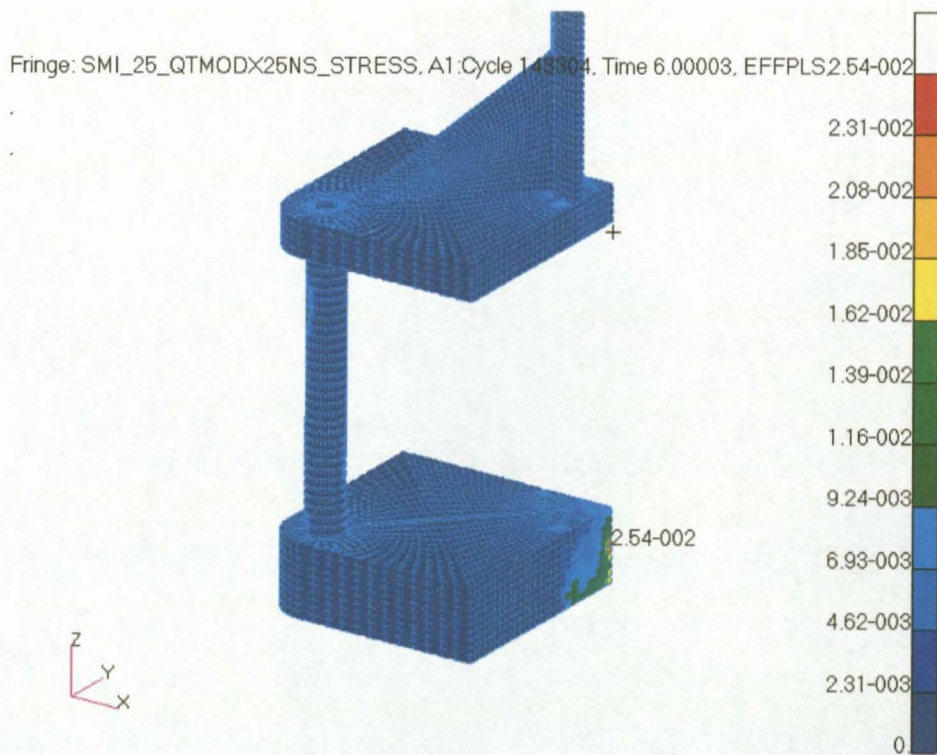
Figure 6.17: A close-up of Figure 6.16, 29.5 N·s load, 3.5 \mu s duration, 77 mm burn diameter.
