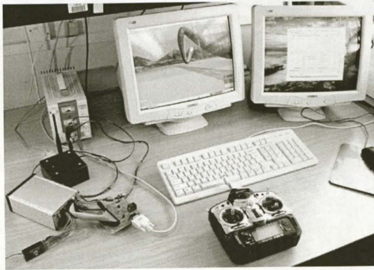
Figure 7.1: Hardware in the Loop Simulation Setup
