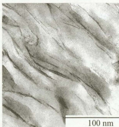
Fig. 6. 16: TEM image for poly(S-co-BA)-AMPS at 15 % clay loading.
