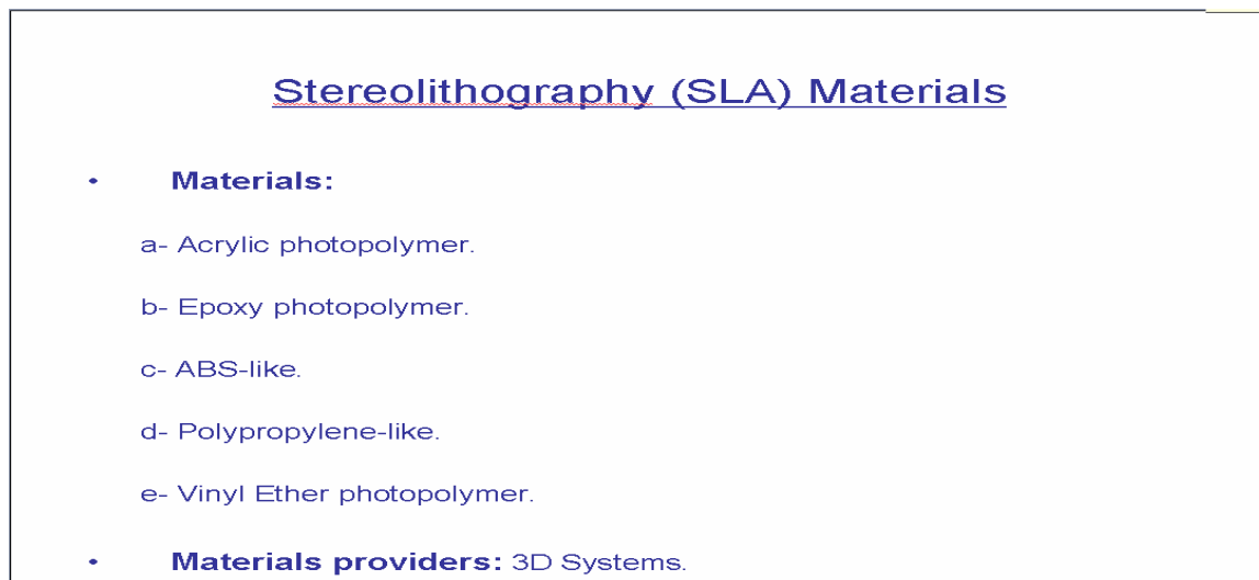
Figure 40 Stereolithography (SLA) materials
