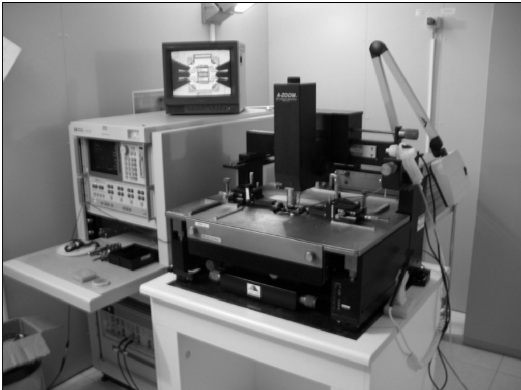
Figure 2.4 The HP8510C VNA was used to measure the linear S-parameters of the on-wafer GaN HEMT devices at IMEC.
