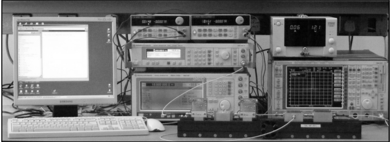
Figure 3.12 A photograph of the IMD system used for test fixture measurements at the University of Stellenbosch to extract the higher order current derivatives of the CFY-30 GaAs FET.
