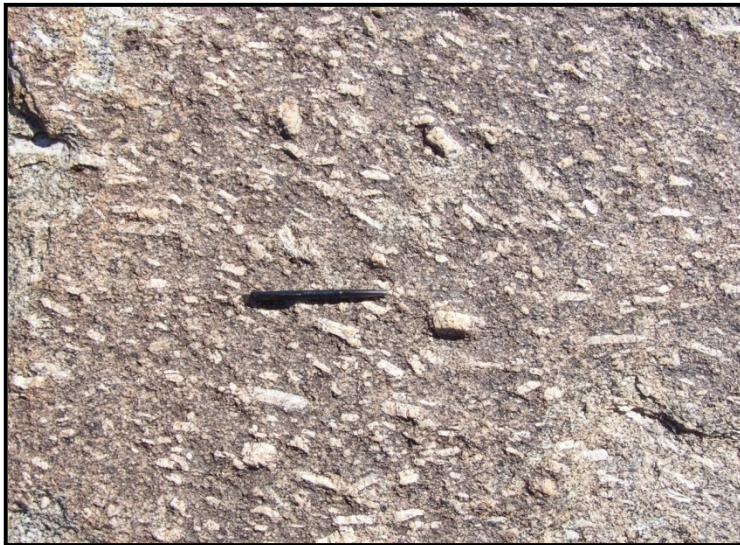
Figure 5.11 , biotite-rich megacrystic Stinkbank granite with a magmatic fabric defined by the orientation of K-feldspar megacrysts. The magmatic fabric trends approximately NE-SW.
