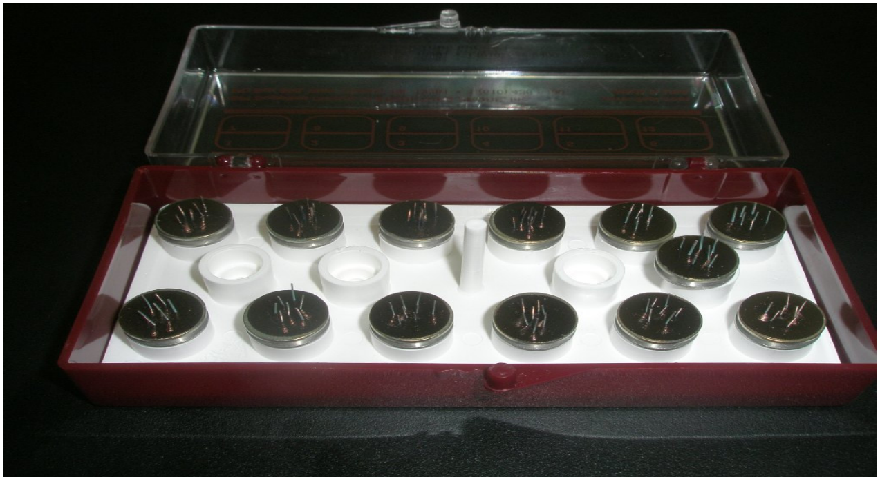
Figure 4-5: Photograph of hollow-fine fibres mounted on stubs for SEM analysis.
