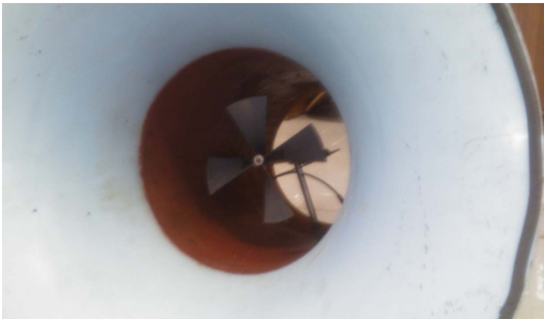
Figure A.1 Propeller anemometer in casing-bellmouth assembly
