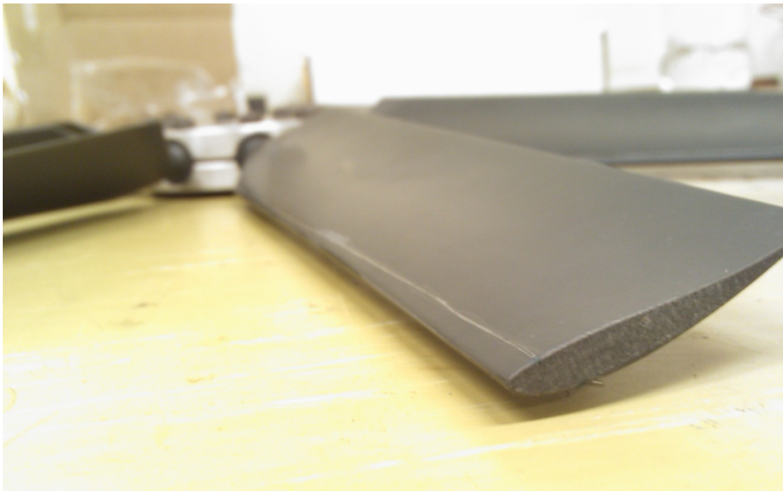
Figure 3.23 Trip wire (0.3 mm fishing line) 'painted' to blade surface
