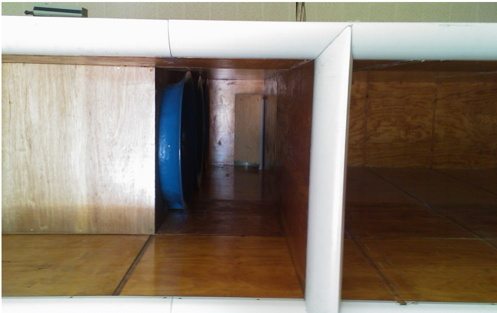
Figure 4.23 Corner chamfer for 'lowest' platform height setting
