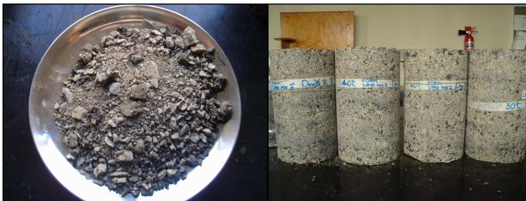
Figure 6.8 Laboratory foam bitumen mixes
