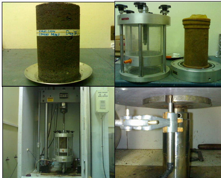
Figure 6.14 Testing of briquettes using laboratory MTS setup and external LVDT
