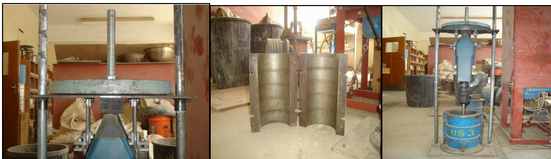
Figure 6.9 Laboratory vibratory compaction protocol using Bosch hammer (Kelfkens, 2007)
