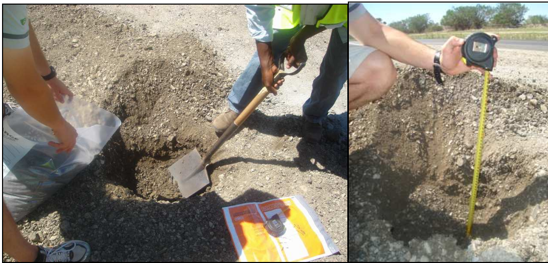
Figure 5.6 Collection of moisture samples on site during and after construction
