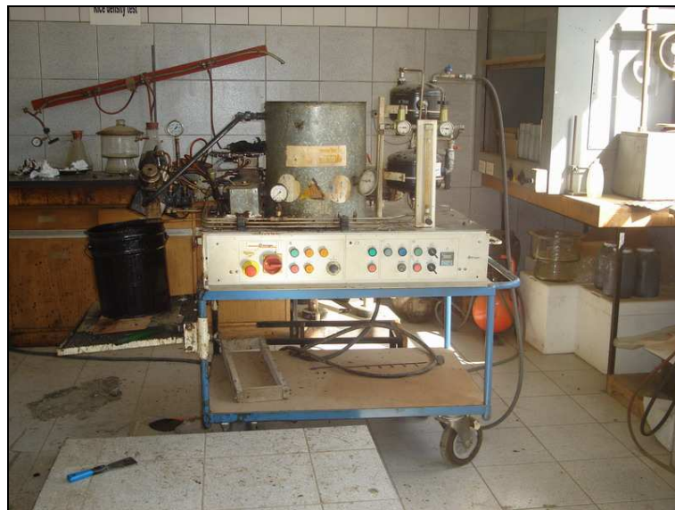
Figure 6.7 Laboratory WLB10 foam plant machine used for BSM-foam
