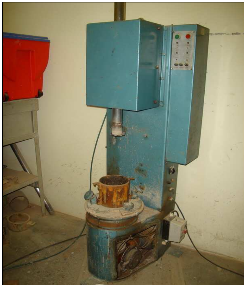
Figure 5.4 Standard Proctor compaction machine at Stellenbosch University
