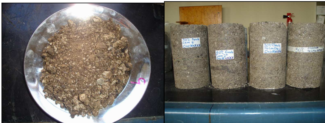
Figure 6.5 Laboratory bitumen emulsion briquettes
