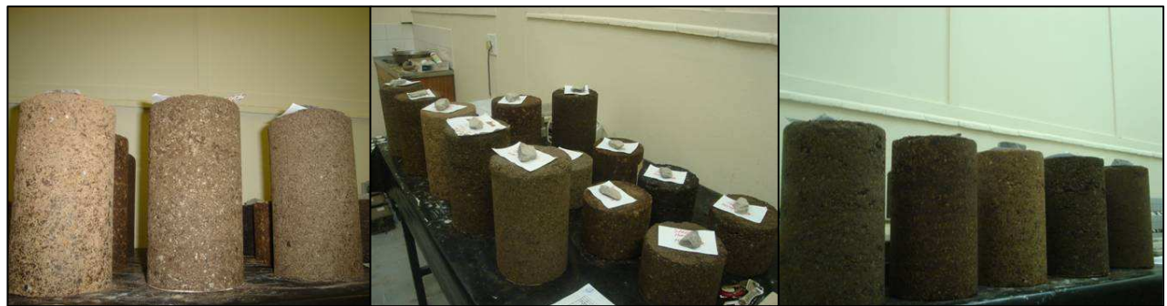
Figure 4.3 Long term curing of crushed rock, ferricrete gravel & sand samples
