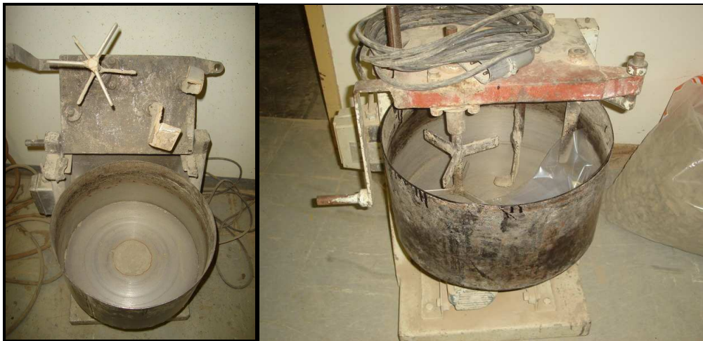
Figure 6.4 Laboratory pugmill mixer used for BSM-emulsion
