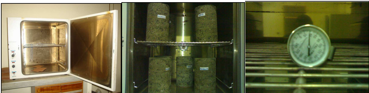
Figure 6.11 Laboratory draft oven curing environments
