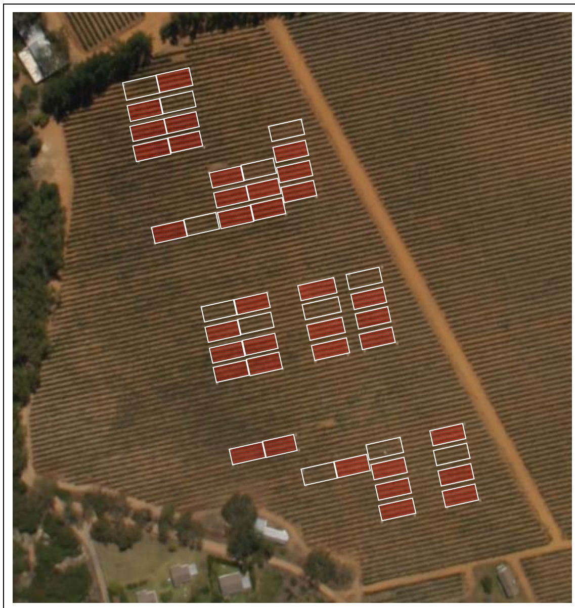
Figure 3.6 Aerial image that indicate the plots where soil water content was measured at 0.3 m depth intervals to a depth of 1 m using a neutron probe. Gravimetric soil moisture content was also measured at the same plots at a depth of 30cm, 60cm and 90cm.
