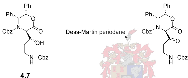
Figure 4.7: Oxidation of the hydroxyl-group of 4.5b to form the corresponding ketone using Dess-Martin periodinane
