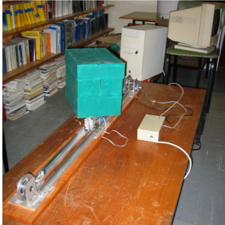
Figure 7.1: The LED-fitted target (box) mounted on the computer-controlled sliding rail
