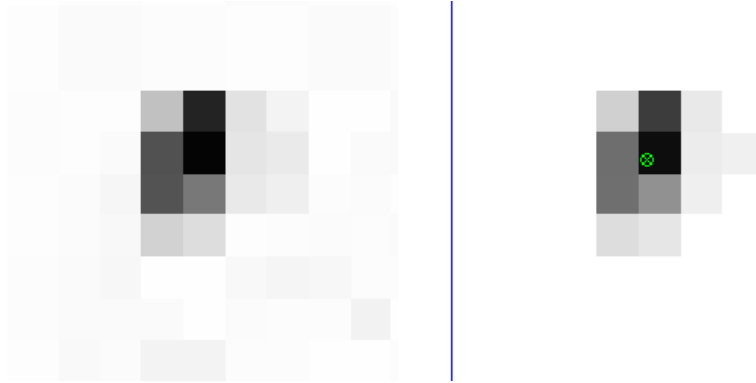
Figure 5.2: An example of a single 2D feature point before and after processing. Thresholded result with "centre of intensity" indicated.
