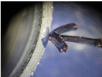
Figure A20.3 Predicted fracture origin
