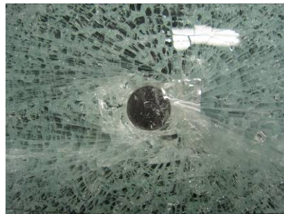
Figure A14.4 Actual fracture origin
