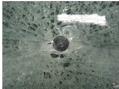
Figure A24.4 Actual fracture origin
