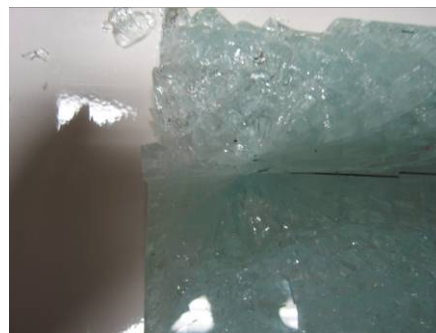
Figure A4.4 Actual fracture origin
