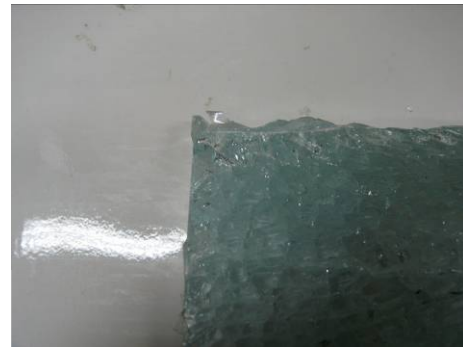
Figure A3.4 Actual fracture origin
