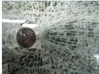
Figure A7.4 Actual fracture origin
