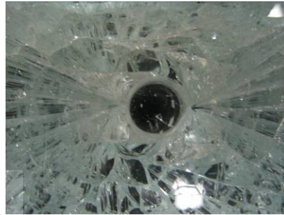
Figure A21.4 Actual fracture origin
