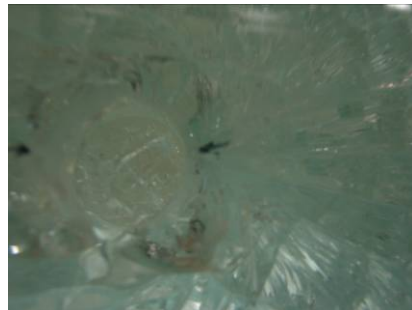
Figure A10.2 Hole in panel
