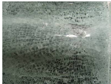
Figure A29.2 Actual fracture origin
