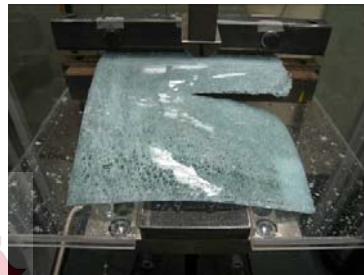
Figure A34.2 Actual fracture origin
