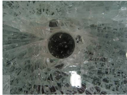
Figure A25.4 Actual fracture origin
