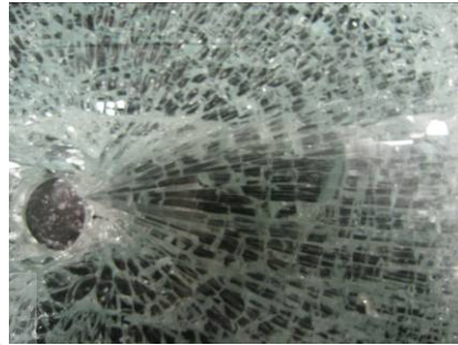
Figure A9.4 Actual fracture origin
