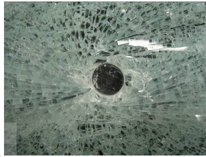
Figure A13.4 Actual fractured origin
