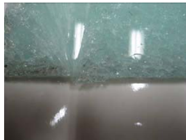
Figure A2.4 Actual fracture origin
