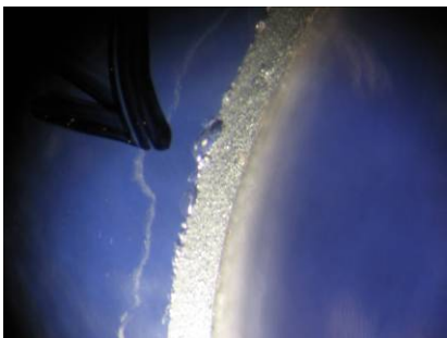
Figure A12.3 Predicted fracture origin
