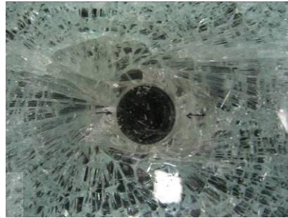
Figure A15.4 Actual fracture origin
