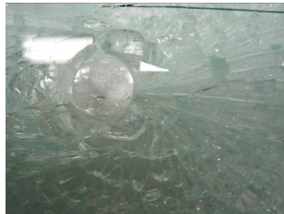
Figure A6.4 Actual fracture origin
