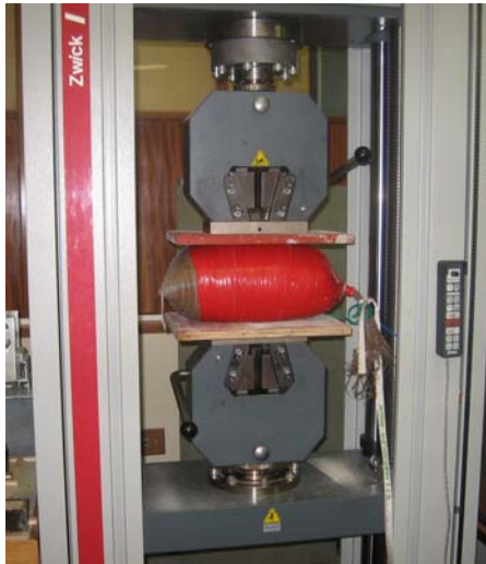
Figure 6.14. Determination of stiffness of test impactor
