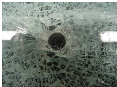
Figure A18.4 Actual fracture origin
