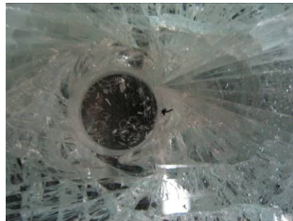
Figure A26.4 Actual fracture origin
