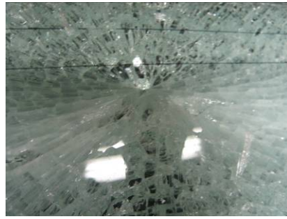
Figure A30.2 Actual fracture origin
