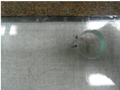
Figure A17.3 Predicted fracture origin
