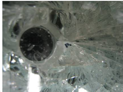
Figure A19.4 Actual fracture origin
