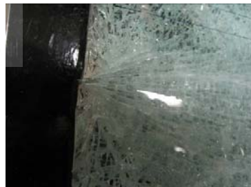
Figure A35.2 Actual fracture origin
