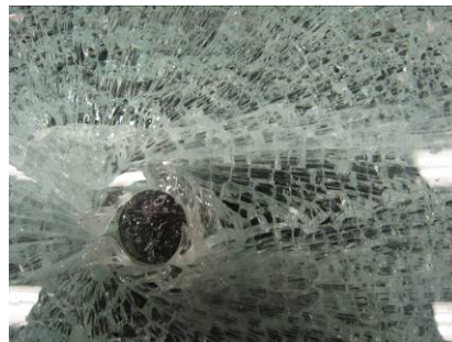
Figure A8.4 Actual fracture origin
