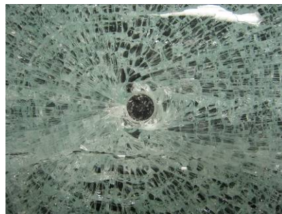
Figure A12.4 Actual fracture origin
