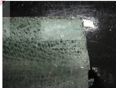
Figure A28.2 Actual fracture origin
