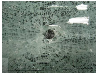
Figure A11.4 Actual fracture origin
