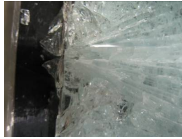
Figure A37.2 Actual fracture origin
