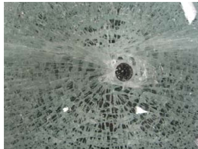
Figure A22.4 Actual fracture origin
