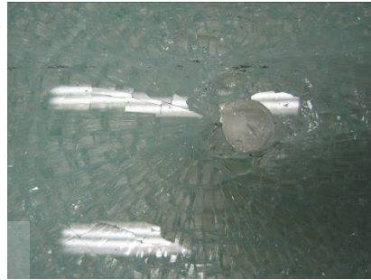
Figure A5.4 Actual fracture origin
