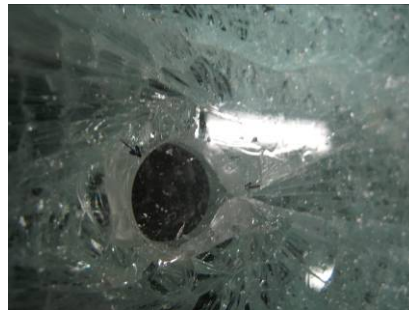
Figure A16.4 Actual fracture origin
