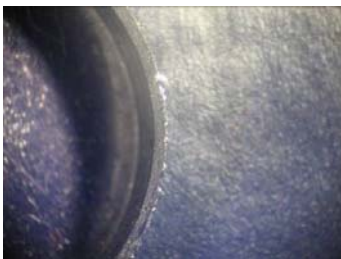
Figure A2.3 Predicted fracture origin
