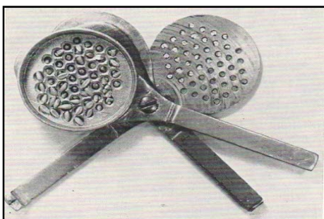
Figure 2.3 The Farinator device used to determine the vitreousness percentage of wheat (Simmonds, 1974).
