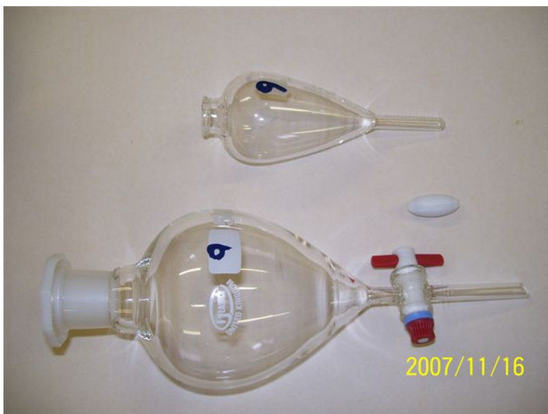
Separating funnel, 35 mm egg-shaped magnet and calibrated pear-shaped flask.
