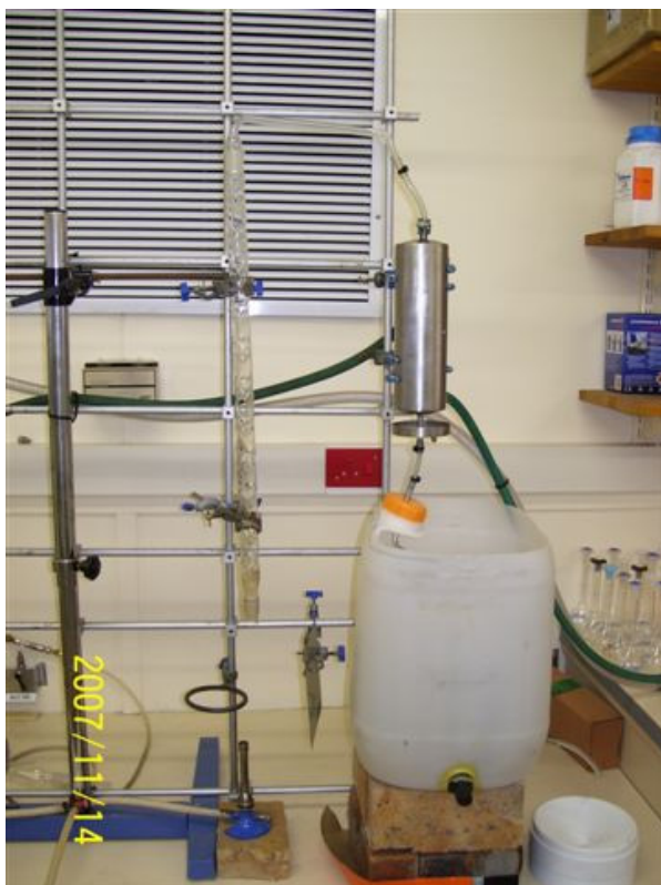
Distillation apparatus with 60 cm fractionating column.
