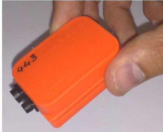
Figure 2-23 – Size of typical Inertial sensor, Xsens
