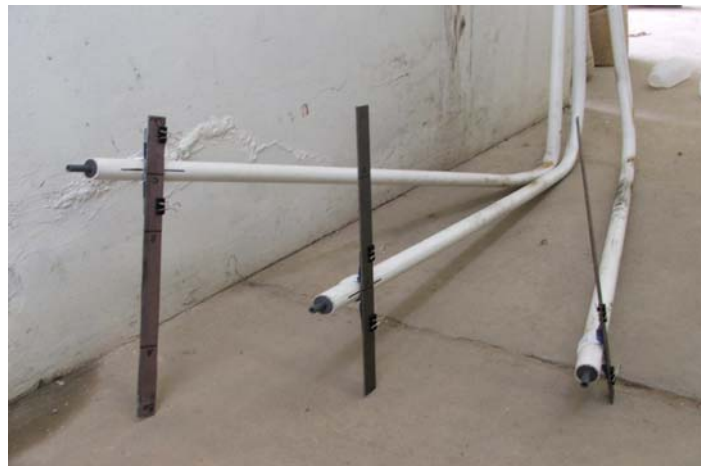
Figure 6-7: The suspended sediment samplers at their three different measuring depths
