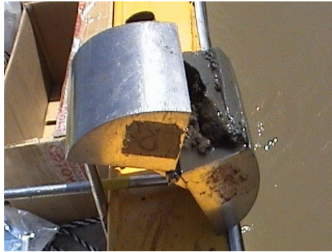
Figure 8.3-4: The grab sediment sampler with a typical load of cohesive sediment from Vaal Reservoir
