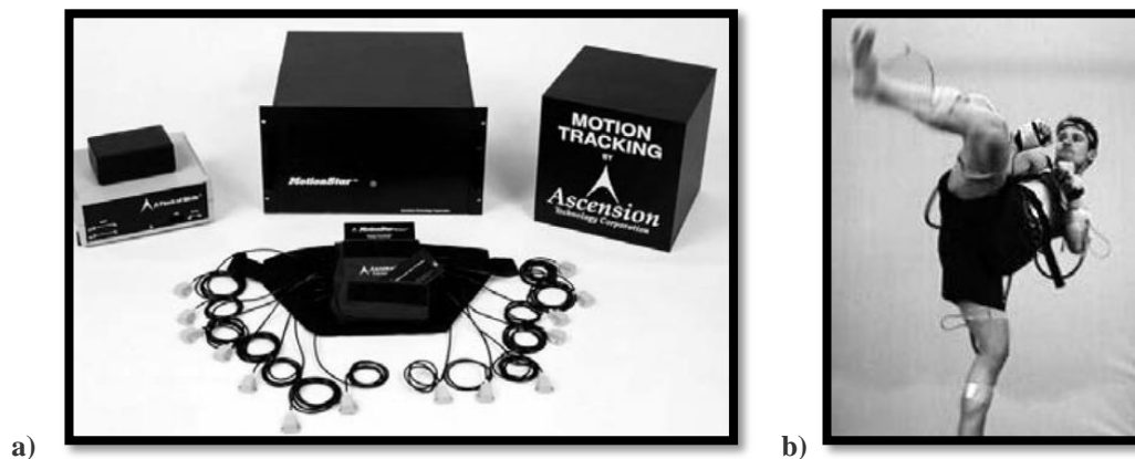
Figure 6: Electromagnetic motion capture system Source: Ascension Technology Corporation (2007)
