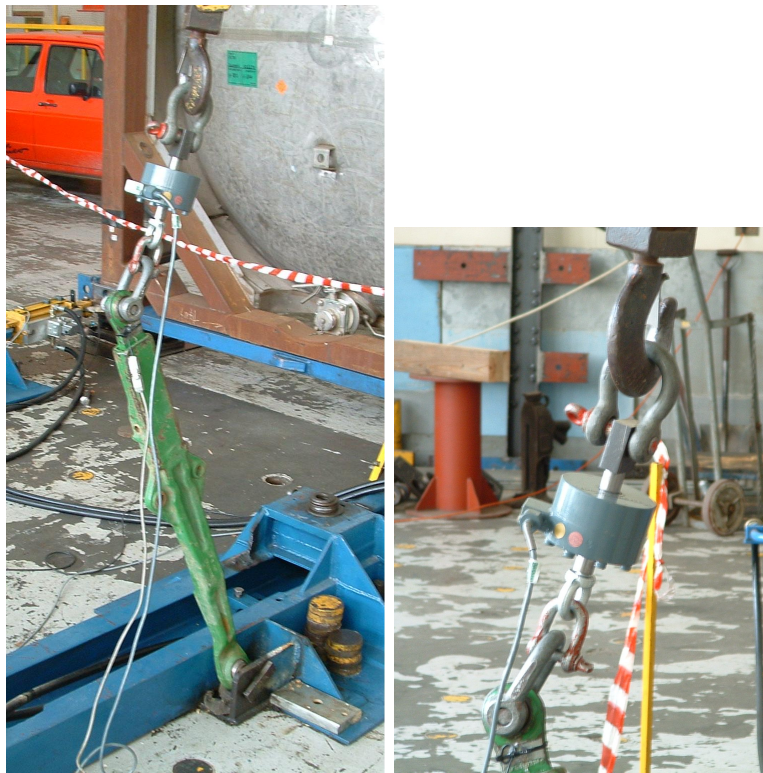
Figure B.1.2: Calibration setup and load cell connection
