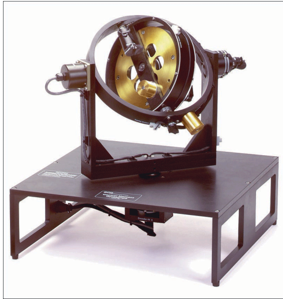
Figure 1.2: A three-degree-of-freedom gyroscope [26]
