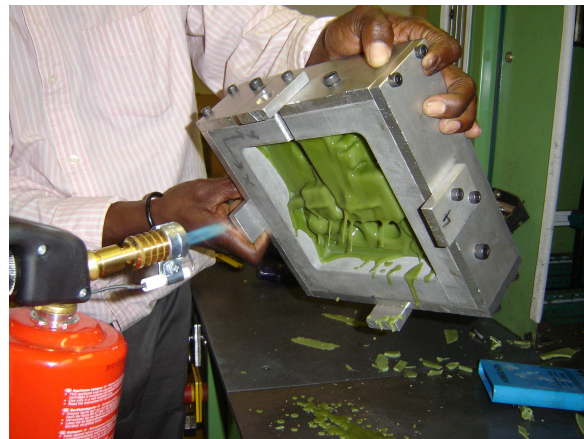
b. Pattern Melted with Butane Flame
