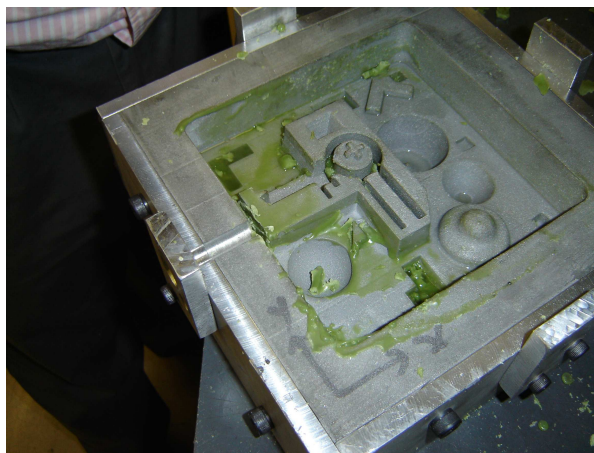
c. Alumide Cavity Cleaned with Trichloroethylene
