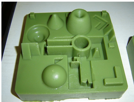
a. Poor Definition on Edges and Points
