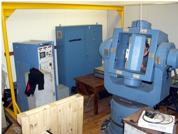
Contravez 3-axis rate table room. The rate table has some electrical problems, but can still be moved manually.
