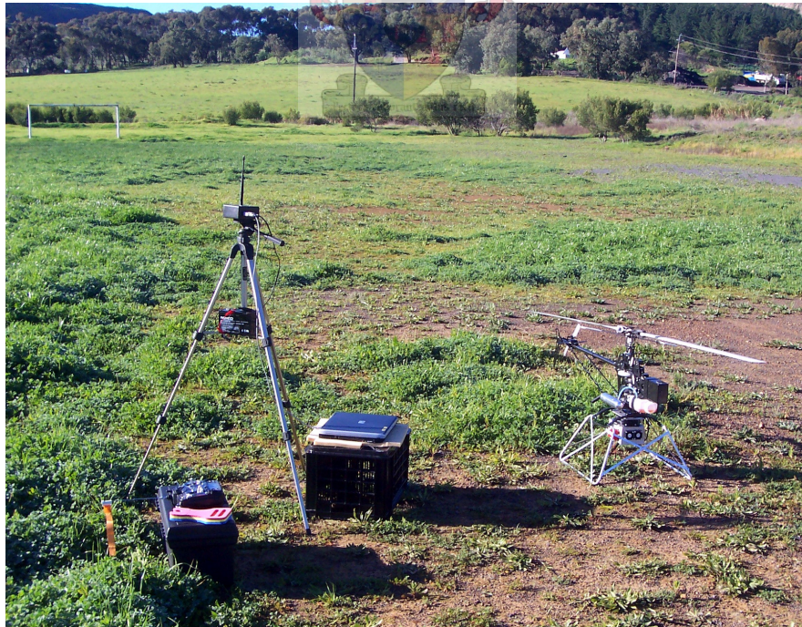
Figure A-10: Flight test equipment: Flight box and transmitter (front, left), AeroComm RF module mounted on a standard camera tripod, and Laptop for ground-station software.
