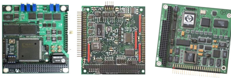
Figure 4-2: PC/104 Data acquisition devices. Left to right: Apex STX104 [42], Kontron ADIO128 [49], Octagon DMM-16-AT [53].
