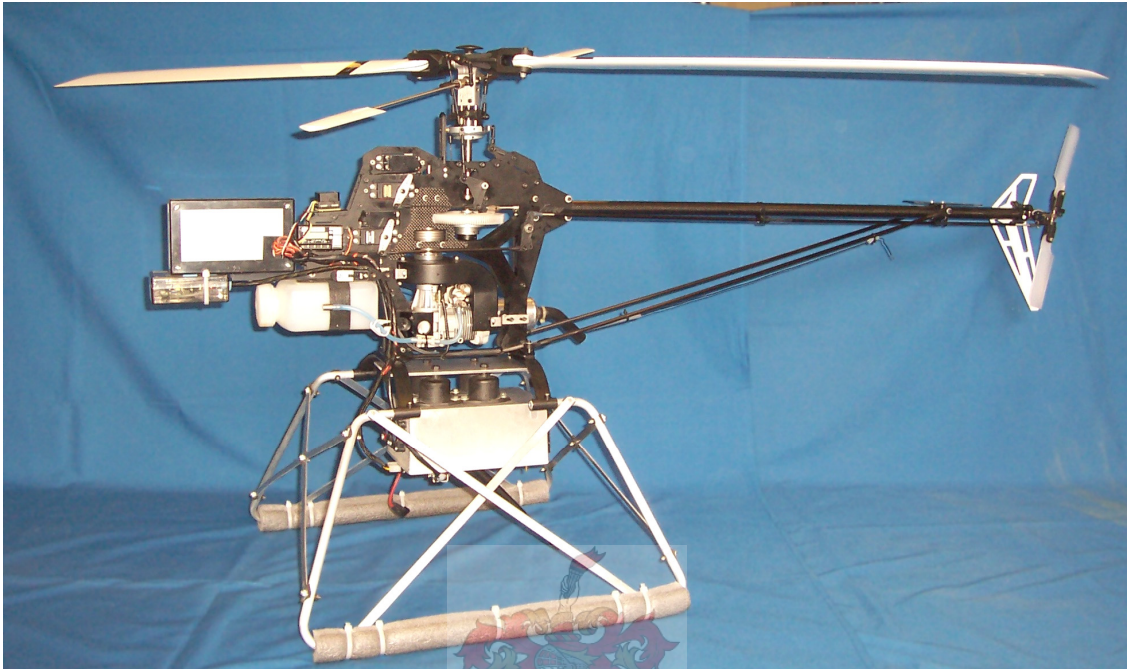
Figure A-5: Modified X-Cell 60 with avionics and extended skids fitted. White vinyl was added to the black nose and tail to make it easier to fly for the pilot. The canopy was removed since it does not affect hover performance and only adds weight.
