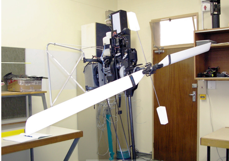
Figure A-9: The X-Cell during measurement of roll inertia. The helicopter was cumbersome to suspend for the torsional pendulum test.
