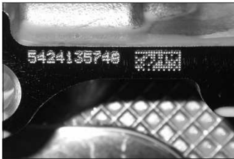
Figure 31: Data matrix encryption on a BMW cylinder head together with the ten-digit, ten-year unique code [48]
