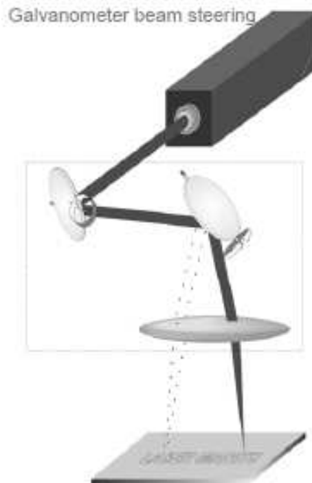
Figure 17: Galvanometer beam steering [30]
