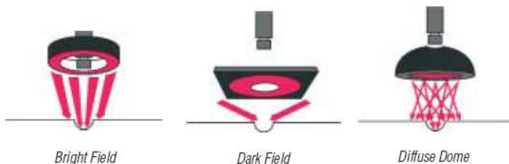
Figure 23: The different types of lighting approaches [25]
