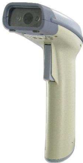
Figure 24: Hand held 2D barcode reader [83]
