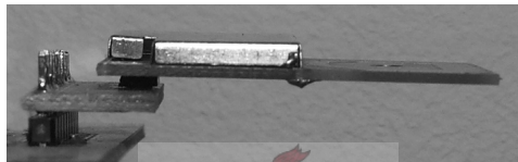
Figure 9.8: nRF2401 connection to 10-pin male header (side view)
