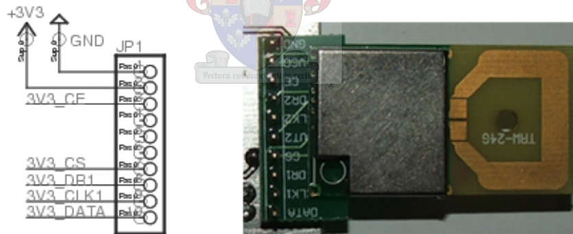
Figure 9.9: Schematic of nRF2401 10-pin male header circuitry and photo of nRF2401 connected to its header.
