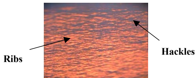
Figure 6.1. Typical ESC surface of sample B after removing soluble fractions (magnification shows area of 50 x 50µm)
