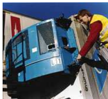
(b) Genset transport [251]. The generator provides electricity to the integral container to which it is attached.
