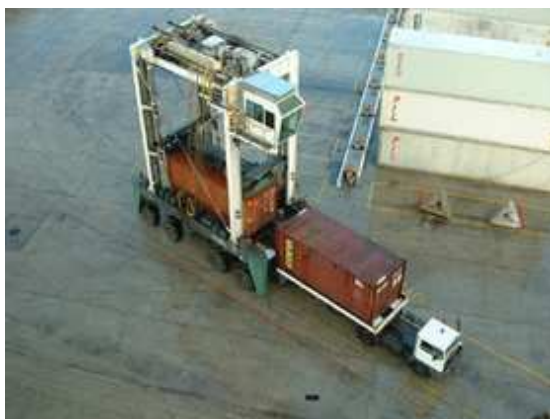
(b) A straddle carrier loading a container onto a bathtub trailer being pulled by a hauler [269].
