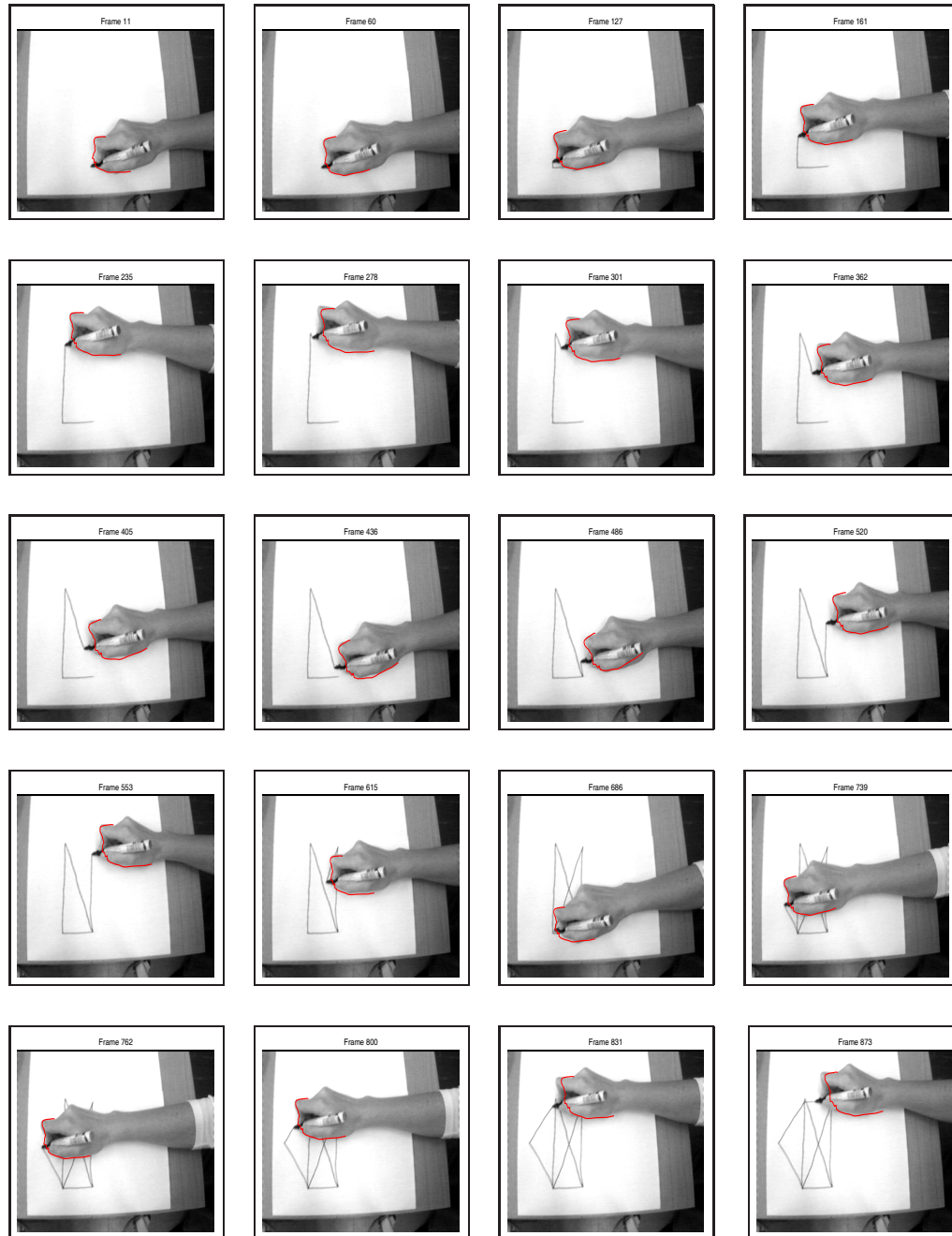
Figure 5.20: Random selection of result frames to indicate the performance of the curve fitting algorithm, when tracking the movement of a hand drawing a picture. The Euclidean regulator was used with \alpha = 0.01 .
