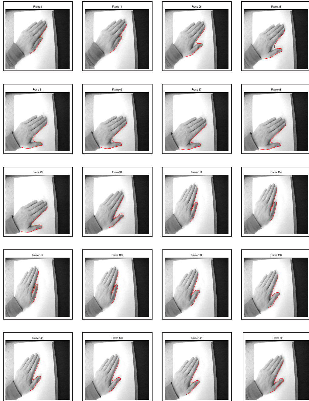
Figure 6.8: Random selection of result frames to indicate the performance of the curve fitting algorithm, when tracking real data with six keyframes and an Euclidean regulator ( \alpha = 0.005 ). Typical deformations are rotation and translation.
