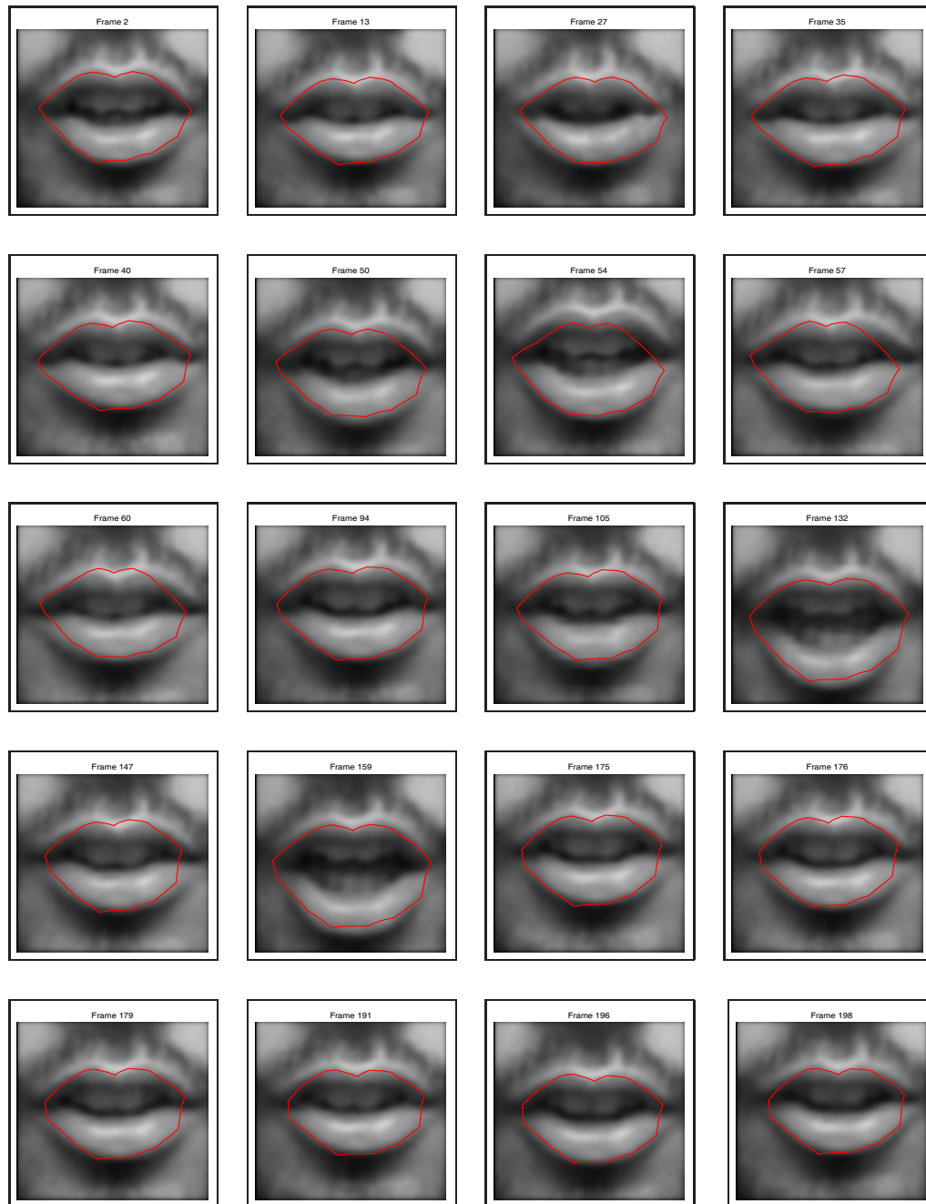
Figure 6.10: Random selection of result frames to indicate the performance of the curve fitting algorithm, when tracking the movement of lips during speech, using keyframes.
