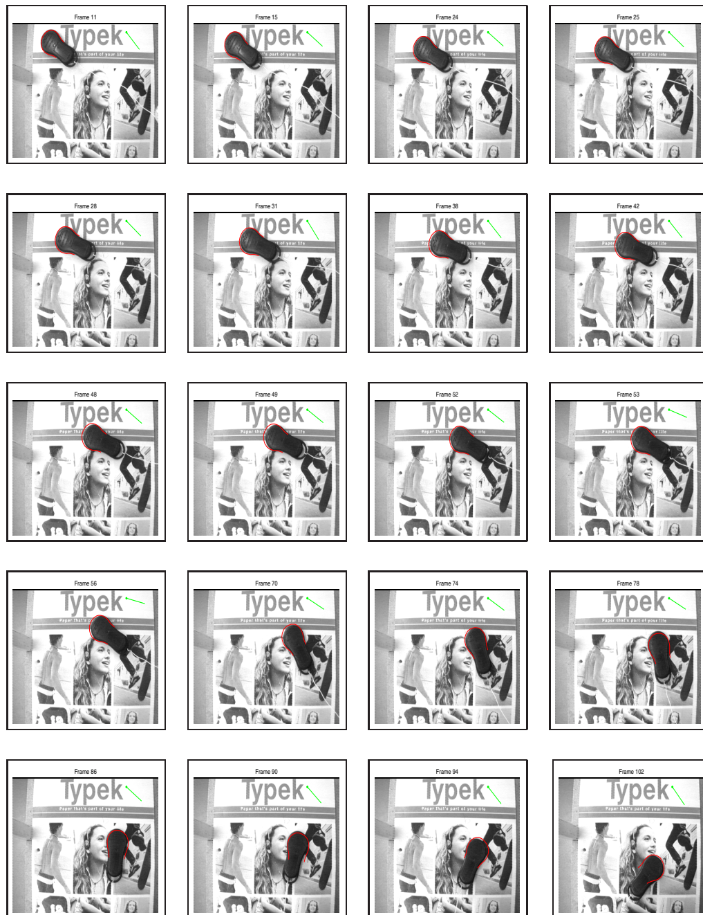
Figure 5.19: Random selection of result frames to indicate the performance of the curve fitting algorithm when the deformation between frames becomes quite big. Tracking is done with an open curve, implementing optical flow as well as scale and rotation limiting.
