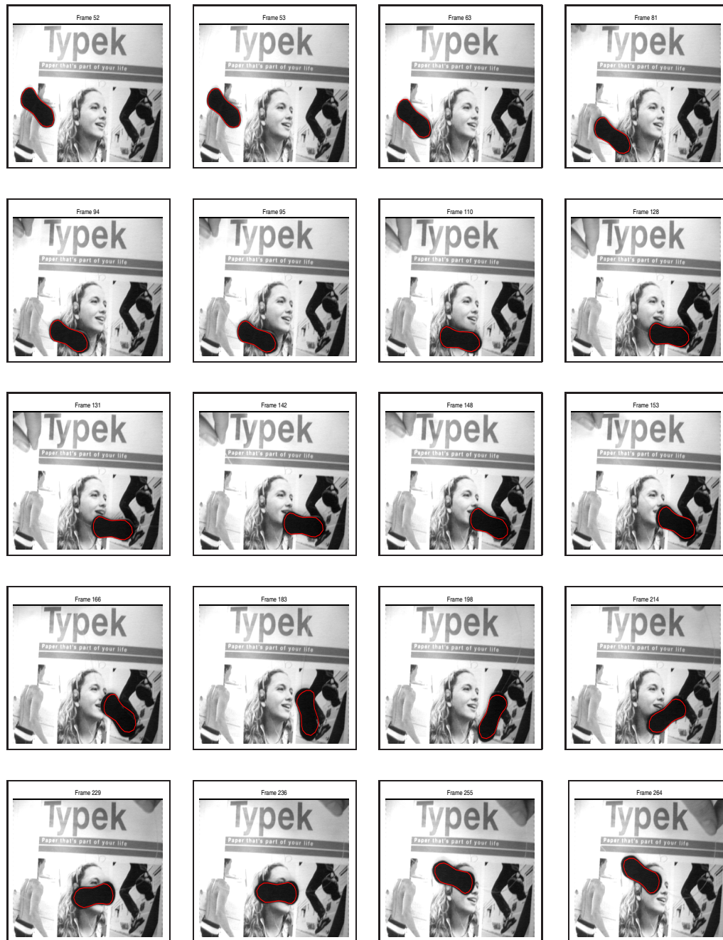
Figure 5.13: Random selection of result frames to indicate the performance of the curve fitting algorithm, when tracking against a cluttered background and limiting scaling and rotation.
