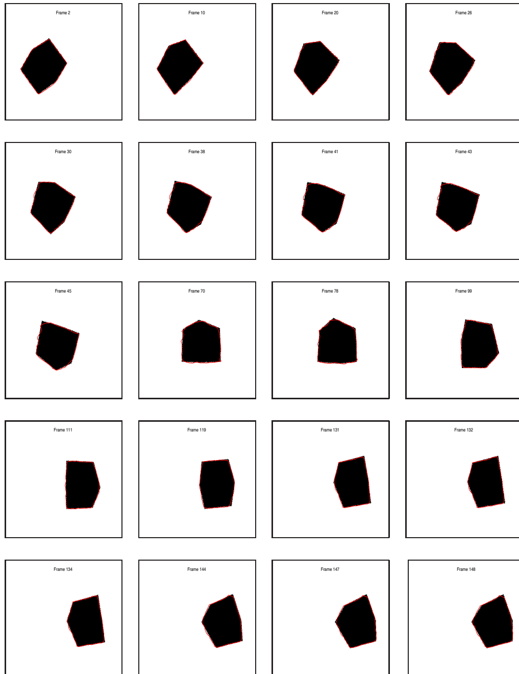
Figure 6.3: Random selection of result frames to indicate the performance of the curve fitting algorithm, when tracking with seven keyframes and an Euclidean regulator ( \alpha = 0.001 ). Deformations are rotation and translation.
