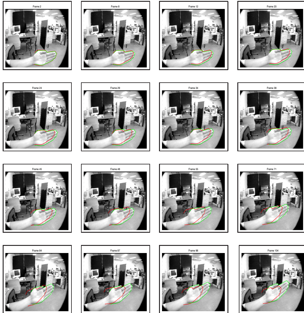
Figure 7.7: Random selection of result frames to compare the performance of the Kalman filter (green) with that of the deterministic filter (red) when applied to a real tracking scenario.
