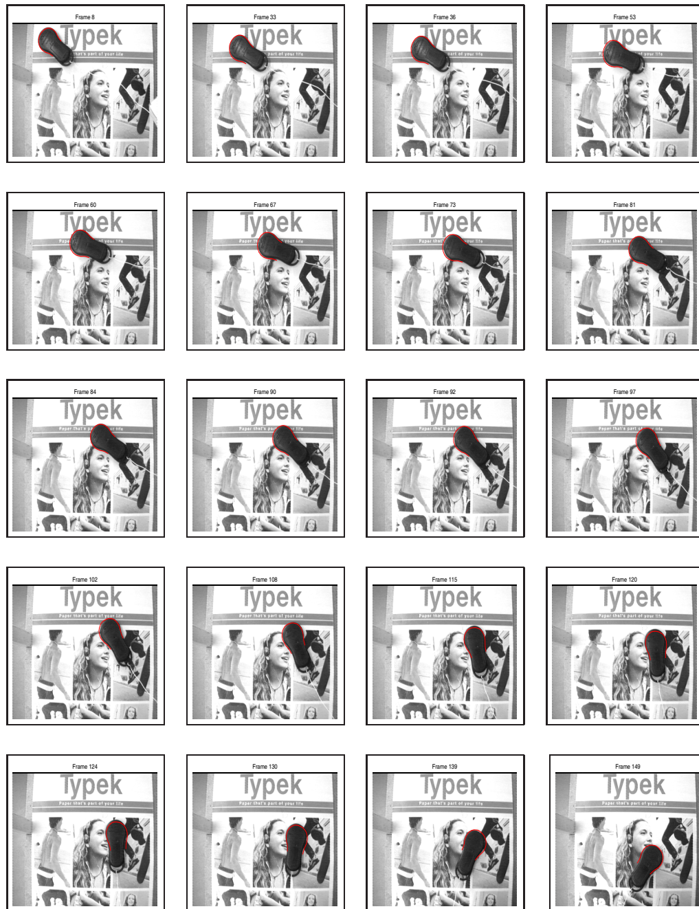
Figure 5.14: Random selection of result frames to indicate the performance of the curve fitting algorithm, when tracking with an open curve against a cluttered background; and limiting scaling and rotation.
