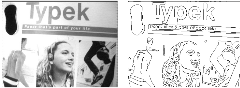
Figure 5.10: A typical image with a busy background and its edge detection result.
