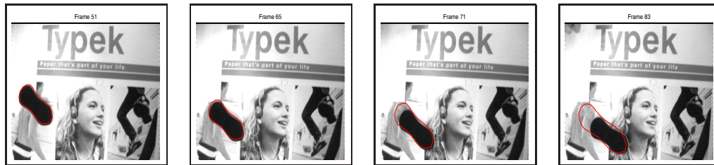
Figure 5.11: Initial tracking with a closed curve against a cluttered background.
