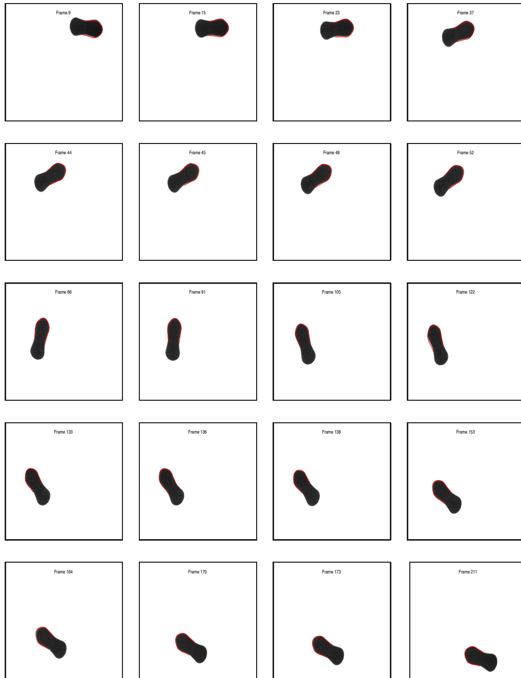
Figure 5.8: Random selection of result frames to indicate the performance of the curve fitting algorithm, when tracking with an open curve, without regularisation.
