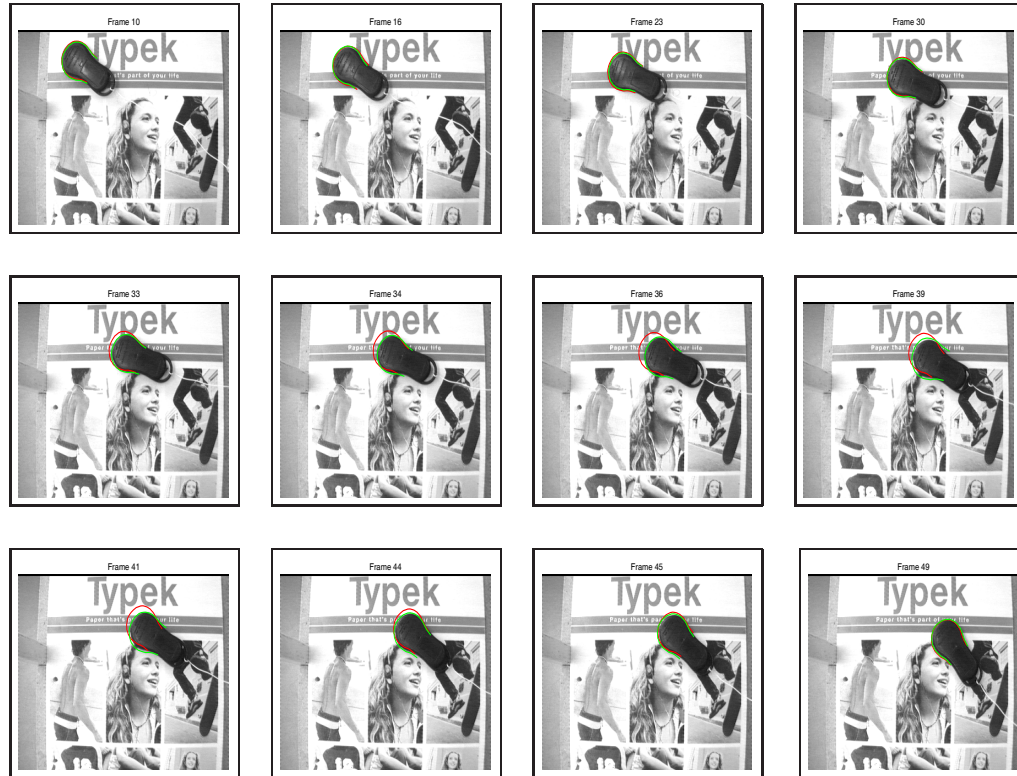
Figure 7.6: Random selection of result frames to compare the performance of the Kalman filter (green) with that of the deterministic filter (red) when applied to a planar affine object that undergoes large deformations.
