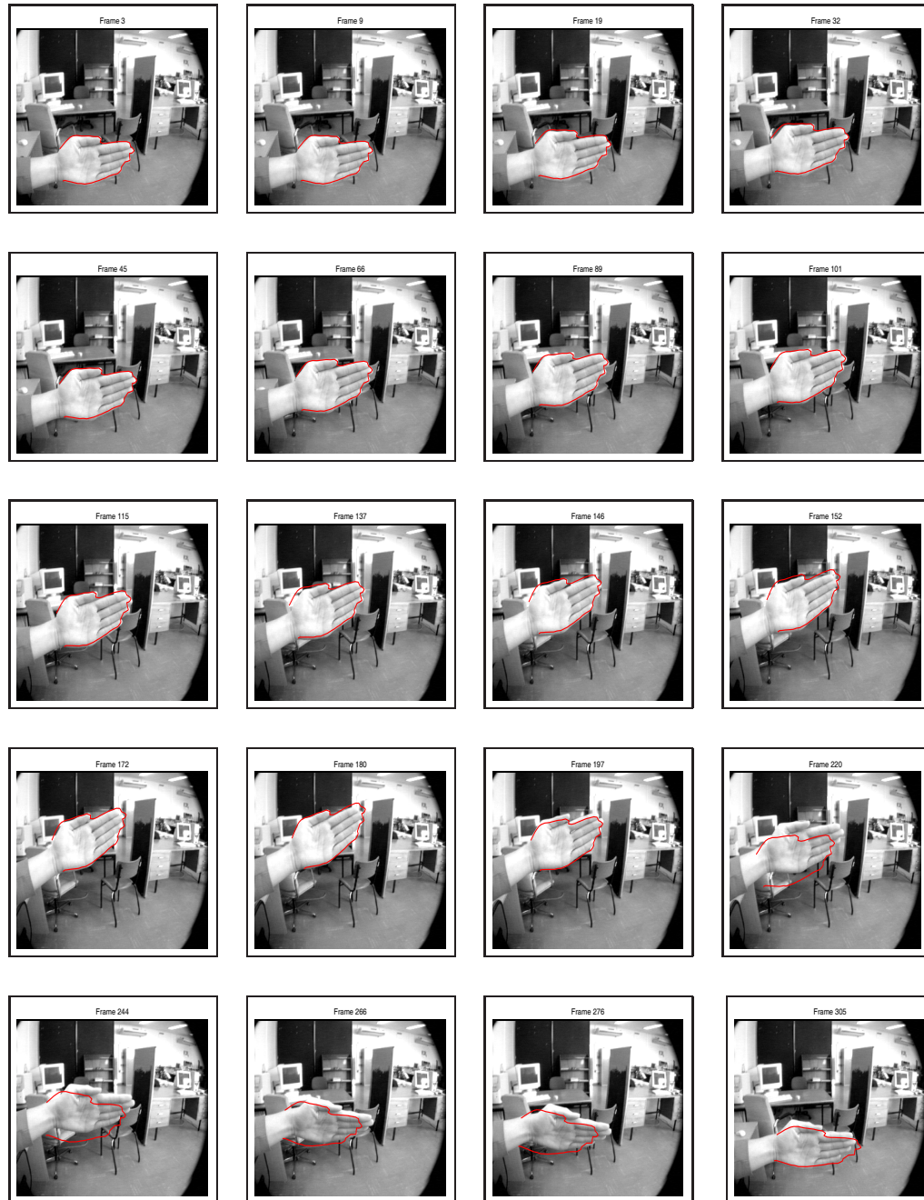
Figure 5.21: Random selection of result frames to indicate the performance of the curve fitting algorithm, when tracking a hand that moves against a realistic background. The Euclidean regulator was used with \alpha = 0.1 .
