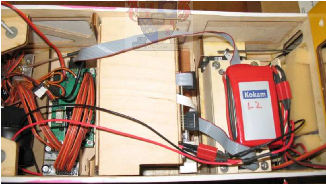
Figure 5.10: Picture of Avionics Mounted inside Fuselage
