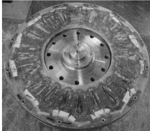
Figure B.2: Phase-grouped non-overlapping winding.
