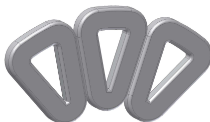
Figure 3.9: 3D drawing of coreless non-overlapping winding.
