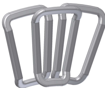
Figure 3.7: 3D drawing of coreless overlapping winding.
