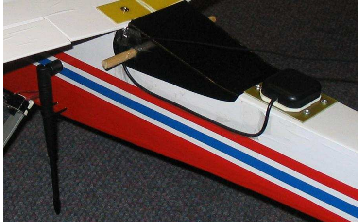
Figure 7.15: Picture of the RF Module Antenna (on the side of the aircraft) and the GPS Receiver Antenna (on the tail of the aircraft)
