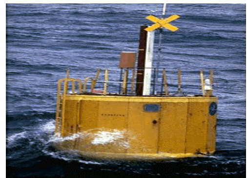
Figure 2-26: Sea trials of IPS buoy
