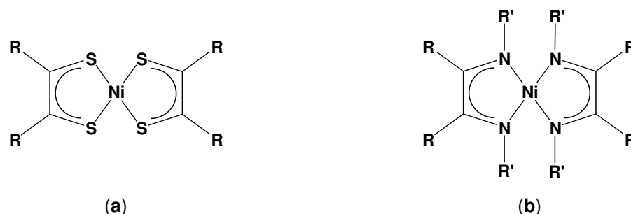
Figure 1.13. Structure of (a) bis(dithiolato)Ni(II) complex and (b) bis( \alpha -diiminato)Ni(II) complex.
