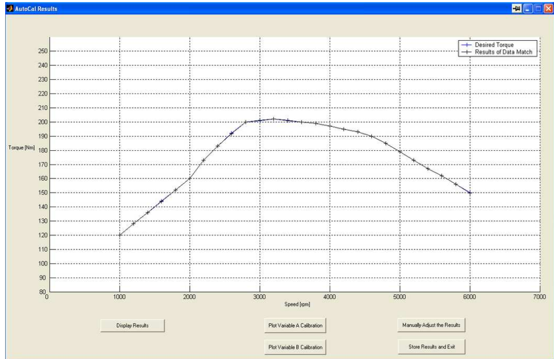
Figure 4.4: Torque match with no constraints enabled.
