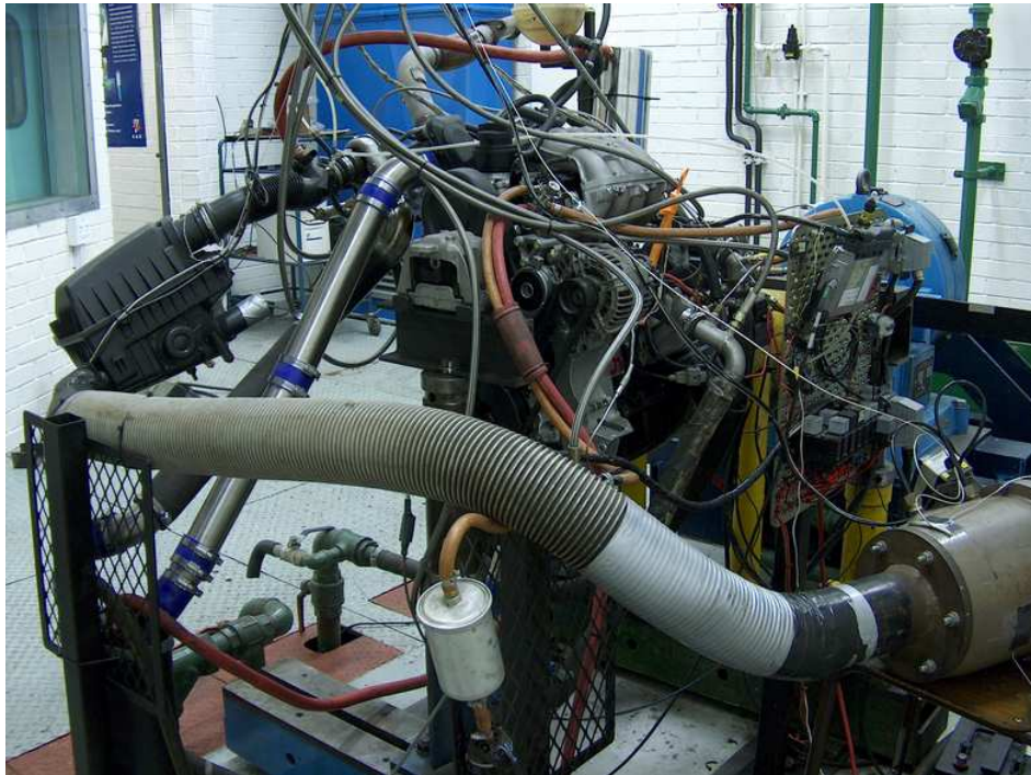
Figure A.5: Air intake components. The laminar air flow meter can be seen on the bottom right-hand side of the picture and the airbox with filter the left-hand side.
