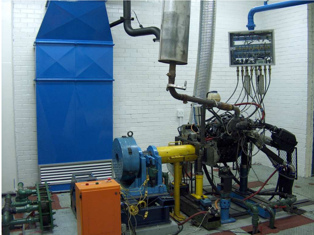
Figure A.9: The test engine installed in the test cell.
