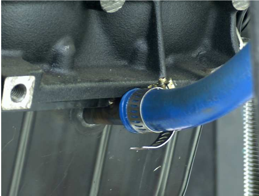
Figure A.3: Oil drain adapter welded into sump with drain pipe from turbo-charger attached.
