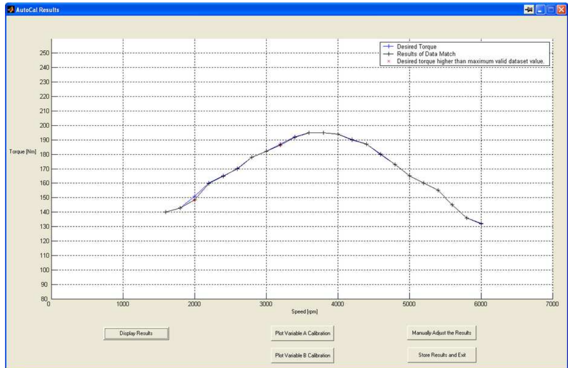
Figure 3.12: The interface used to evaluate the results of the matching process.
