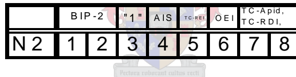
Figure D.1: N2 Byte structure
