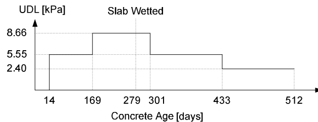
Figure 5-11: Loading History for Slab S1 (Gilbert and Guo, 2005).
