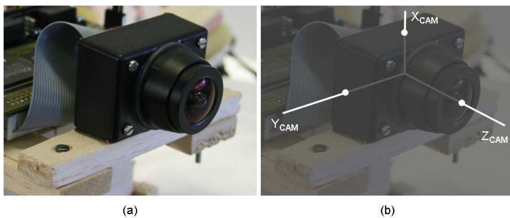
Figure 8.4: (a) The camera sensor unit. (b) The camera axis.
