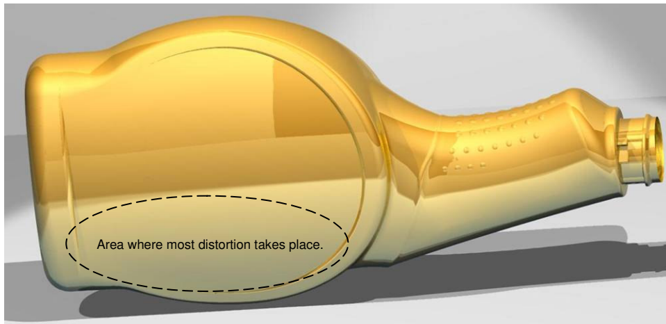
Figure 16: Indication of areas where the most distortion takes place.
