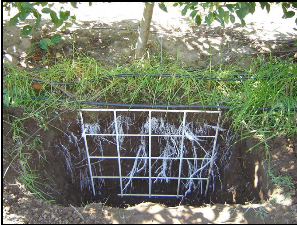
Figure 1. The grid with dimensions of 80 cm wide, 80 cm long and 20 x 20 cm squares that was used to evaluate the concentration of roots vertically distributed through the soil profile as well as horizontally from the dripper.
