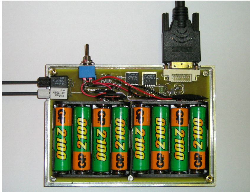
Figure 5.3: Aluminium power box for the batteries.
