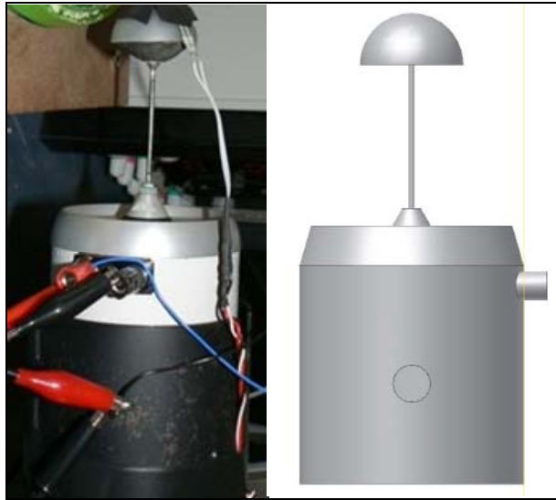
Figure 3.1: Vibrational shaker as implemented
