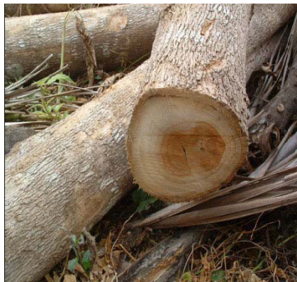
Figure 2. Cross-section of a plantation-grown teak log with its darker heartwood ( Zanin, 2005 ).
