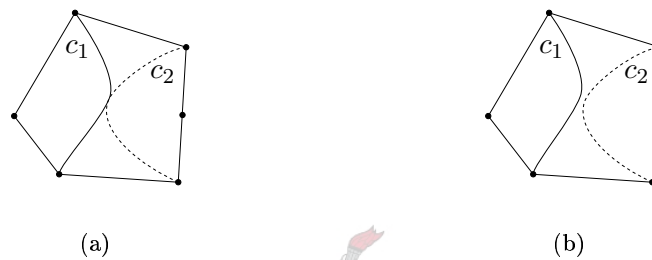
Figure 3.3: Tangential edge intersections may be removed simply by moving curve sections at the intersections far enough apart. The edges c_1 and c_2 have a tangential intersection in (a). This intersection has been removed in (b) by moving the edges away from one another.
